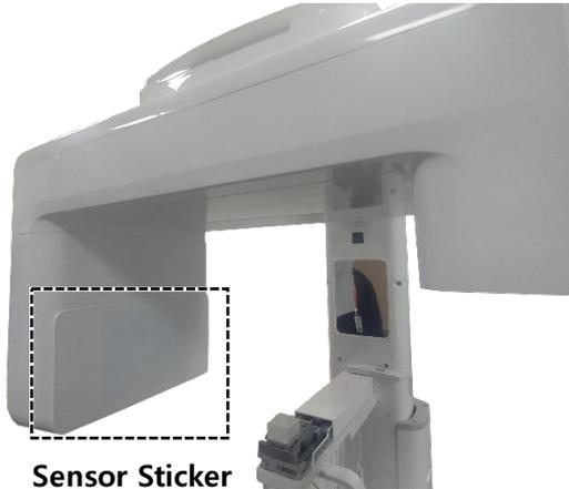
2. Attach your dosimeter to the sensor's active area.
